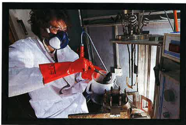
Test case two: the HTC reactor at the Hamburg Technical University now takes just 3 litres of faeces. Under high pressure this turns into coal, ideal as fuel.
