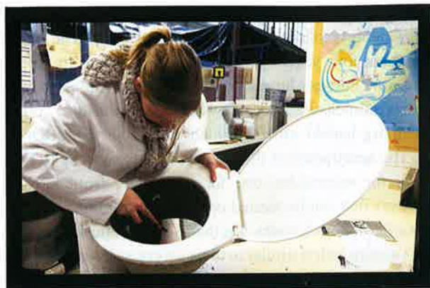
Test case three: the dry toilet of a student—one takes a bucket, cuts out one half of the bottom (for solids) and makes an outlet in the other half.
